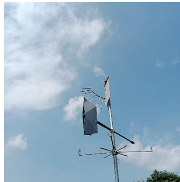
Gambar 1.7 Wind Vane
